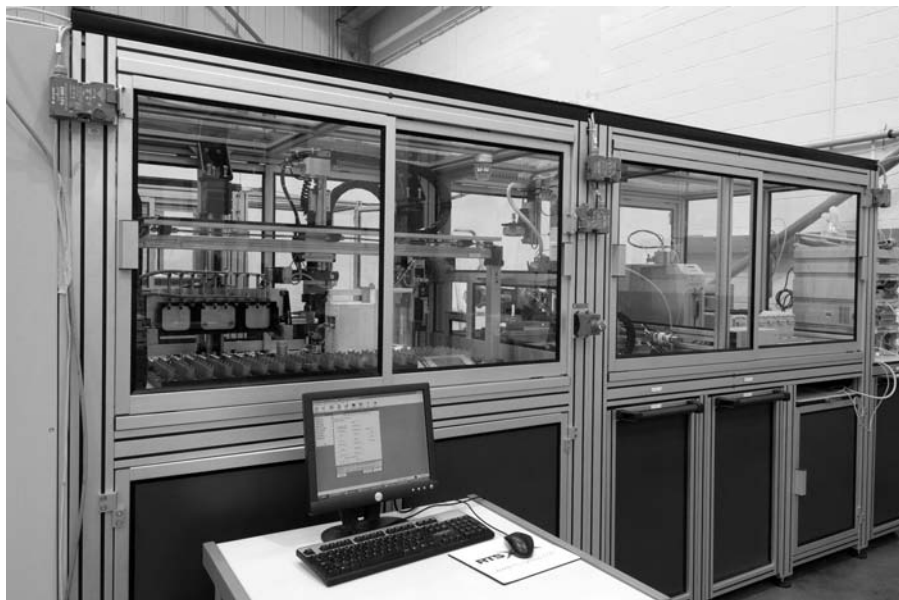
Figure 44.2 Process Master automated inhalation product testing system. (Courtesy of RTS Life Science; www.rtslifesience.com .)
