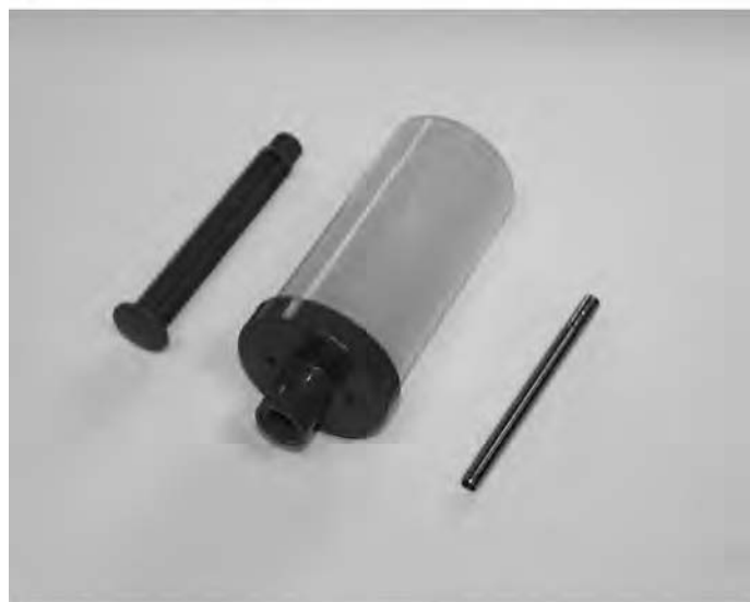
Figure 14.1 Device for capturing breath samples for solvent analysis: (a) schematic; (b) components. (Dyne et al. 1997; illustrations courtesy of Dr J Cocker, Health & Safety Laboratory, Buxton, UK.)
