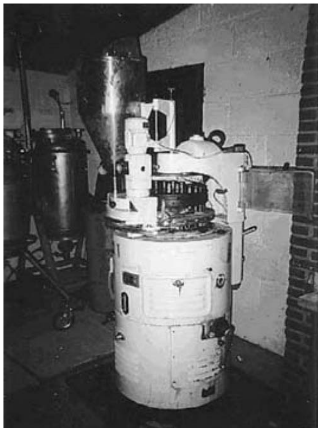
Figure 13.3 Commercial tablet machine used to produce illicit tablets. Reproduced with permission from TICTAC Communications.
