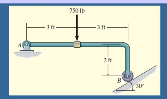
Determine the horizontal and vertical components of reaction on the member at the pin A, and the normal reaction at the roller B in Fig.
