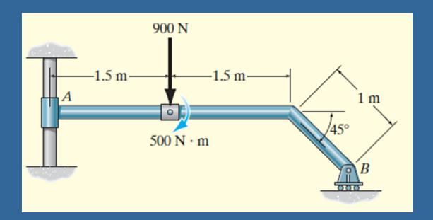
Determine the support reactions on the member in Fig. The collar at A is fixed to the member and can slide vertically along the vertical shaft.
