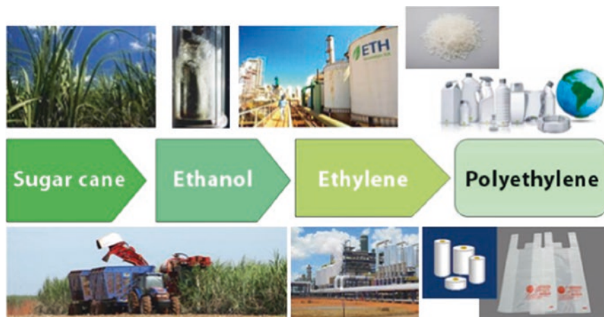
Fig. 11.5 Process for green-PE production ( http://www.sojitz.com/en/news/2012/07/20120705.php )
